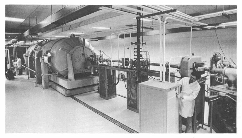
VAN DE GRAAFF tandem accelerator is a powerful research tool for atomic level materials analysis. Ion beams with energies up to 30 million electron volts and velocities up to one-tenth that of light can be obtained with this machine. The beam impacts into a target chamber beyond the back shielded wall. Norman Wing (foreground) and Mark Wilkins (both 5112) ready the accelerator for operation.
